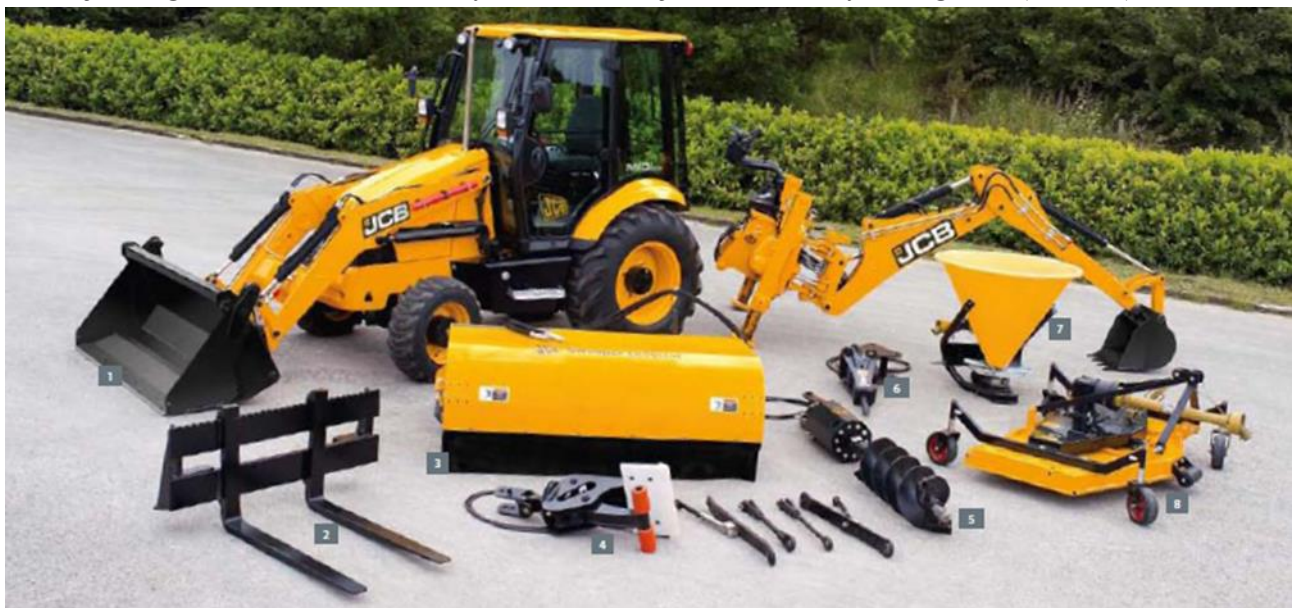
2-rasm. Universal almashinuvchi ishchi jihozli ko‘p maqsadli mashina
