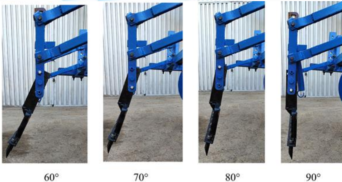
2-rasm. Tishli tekislagichning gorizontga nisbatan o‘rnatilish burchaklari
