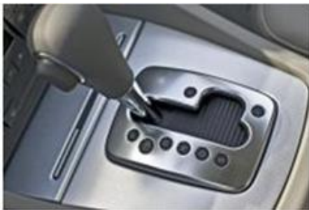
5-rasm. Tiptronik funksiyali AUQni boshqarish richagi
